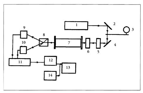
**Figure 1.** A diagram of the system for measuring optical activity of liquid media: (1) He-Ne laser (wavelength 0.63 micrometers); (2,4) reflecting mirrors; (3) shutter; (5,6) polarizers; (7) cuvette with solution; (8) Glan-Thompson prism; (9,10) photodetectors; (11) comparison block; (12) amplifier; (13) oscilloscope; (14) strip-chart recorder.
